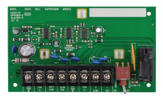
This module is used for wiring connections to remote signaling devices. You can connect up to twelve D192G modules to the same system on compatible control panels. Wiring is supervised for open, short, or grounded circuit faults.
