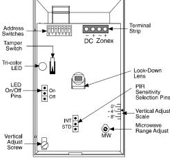
Firmly mount the base to the mounting surface. Return the circuit board to the base and tighten the Vertical Adjust Screw.
