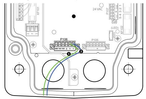
Figure 3.8 Detail of P106 Connections
