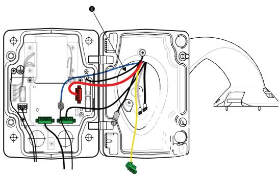
Figure 2.13 IP AutoDome: Pendant Arm connections to Power Supply Box
