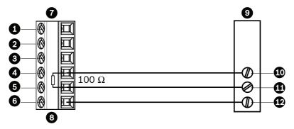
Figure 3.6 Connections for RS485 Operations
