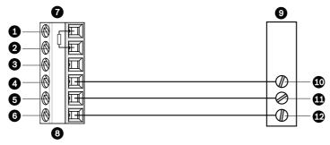
Figure 3.4 Connections for RS232 Operation
