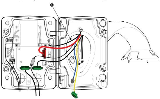
Figure 2.11 Analog AutoDome: Pendant Arm connections to Power Supply Box
