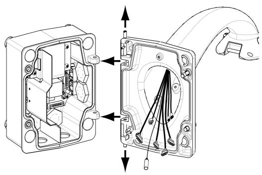
Figure 2.10 Pendant Arm to Power Box Hinge Alignment
