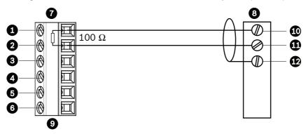
Figure 3.2 Connections for Biphase Operation
