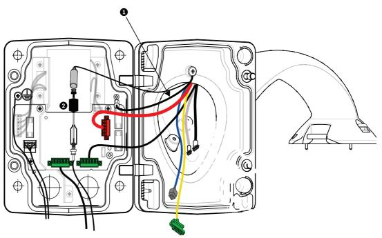
Figure 2.12 600 Series AutoDome: Pendant Arm connections to Power Supply Box
