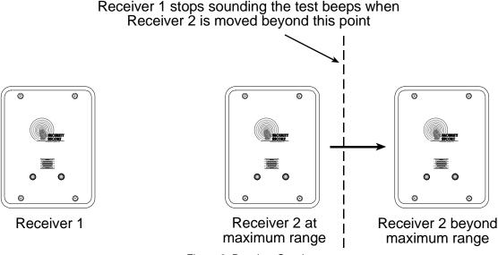
Figure 2: Receiver Spacing
