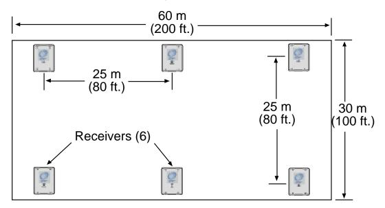
Each floor would require 6 Receivers, resulting in a total of 24 Receivers to protect this building.
