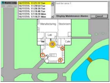
Figure 40: Maintenance "Alarm" With Signal Levels Shown in Icons
