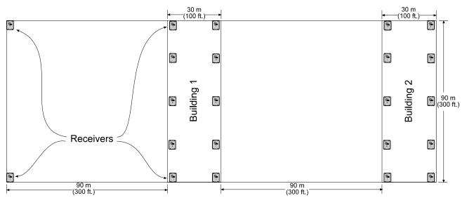
To estimate the number of Receivers, assume a maximum Receiver spacing of 90 m (300 ft.) between Receivers, in both directions, for Receivers that are not within 30 m (100 ft.) of a building with inside coverage. Receivers within 30 m (100 ft.) of a building should be spaced at the spacing of Receivers in the building (spacing the outside Receivers at a somewhat larger spacing is acceptable in most cases).
