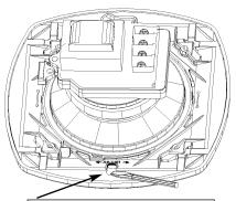
Adjust brightness by using small flatblade screwdriver to turn dial. Displayed number will be candela selected.
