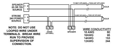
\*MAX. WIRE DISTANCE (IN FEET) = PANEL VOLTAGE - DEVICE MINIMUM VOLTAGE X WIRE CONDUCTIVITY (STROBE ONLY) TOTAL CURRENT DRAW
