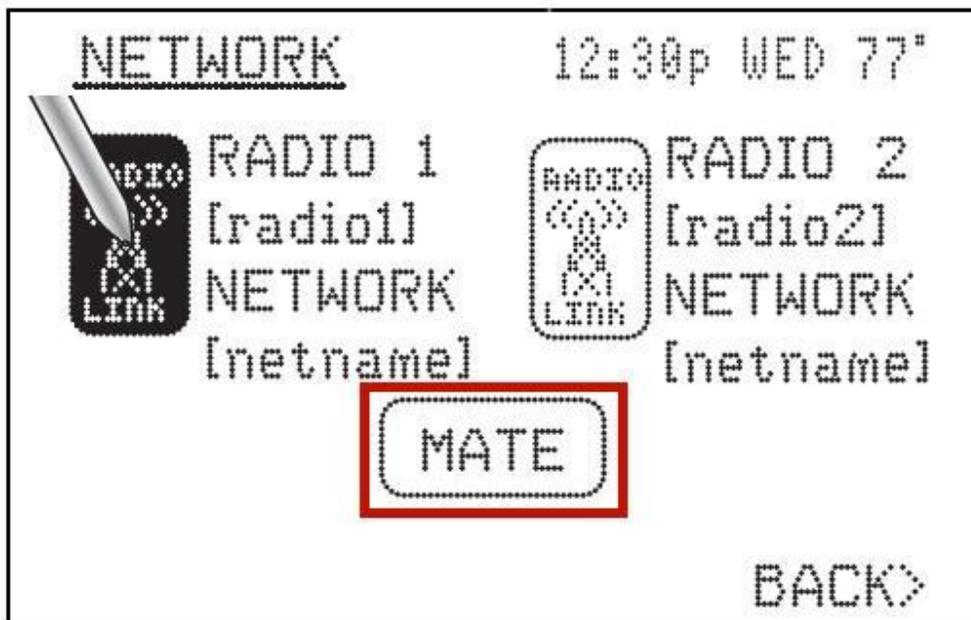
The blinking light on your gateway will go off for a few seconds and then will start blinking again to show the thermostat was paired to it, then return to blinking slowly. The CT80 will display the name of your network to show it was paired.
