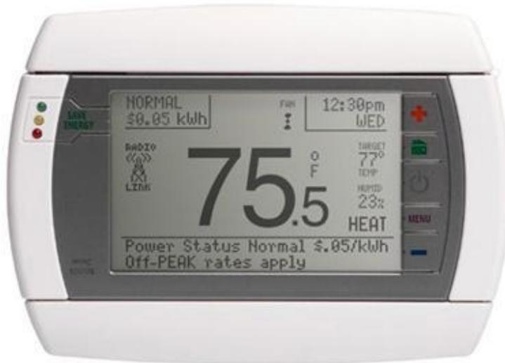
The CT80 can control multiple stages of heating and cooling for energy efficiency, and up to 7 independent periods of climate control per day. This can be a real convenience that saves you money in little ways that add up to big ways.
