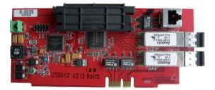
The FPE-1000-NF Fiber Optic Networking Card provides two fiber optic ports for in/out peer-to-peer communication and one additional Ethernet port for communication with the Ethernet and wired cards, for IP reporting, or for browser-based panel/network programming.
