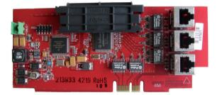
The FPE-1000-NE Ethernet Networking Card provides two Ethernet ports for in/out peer-to-peer communication and one additional Ethernet port for communication with the fiber optic and wired cards, for IP reporting, or for browser-based panel/network programming.
