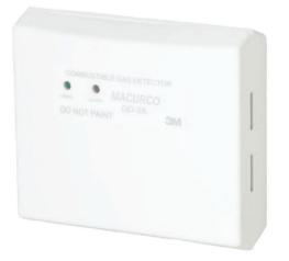
The D382 Combustible Gas Detector (Macurco GD-2A) detects the presence of combustible gases such as propane and natural gas (methane). It is rated by Underwriters Laboratories (UL) to alarm below 25% of the lower explosion level (LEL) of propane or methane.
