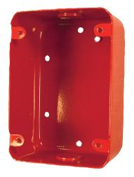
A red cast-metal back box measuring 4.75 in. x 3.25 in. x 2.25 in. (12 cm x 8.3 cm x 5.7 cm) with  $\frac{1}{2}$  inch (12.7 mm) knockouts in the short sides. The back box is UL listed under UL38 and is UL certified for use in Canada. It has been approved by CSFM (7150 1615: 224) and NYC/MEA (382 94 E, Vol. VI).
