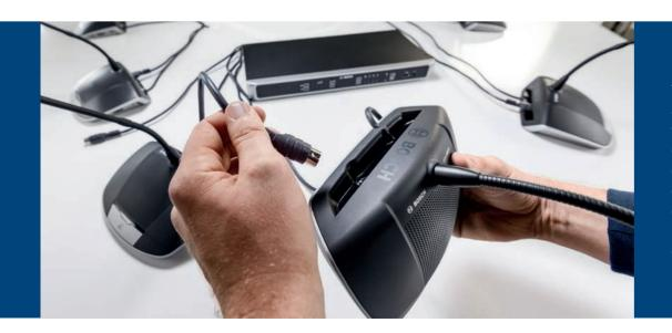
The system is very quick and easy to install. No training or additional equipment is needed: the discussion devices are directly plugged into the control unit via a simple 'daisy chain' cable connection.
