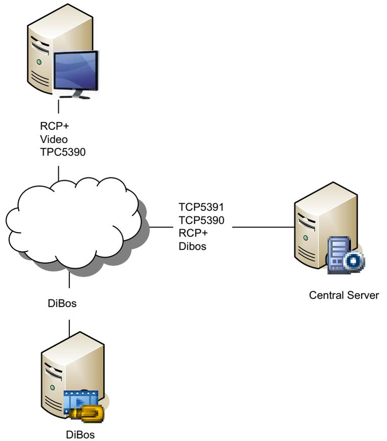
**Figure 6.6** Open ports for a DiBos recorder connected to Bosch VMS
