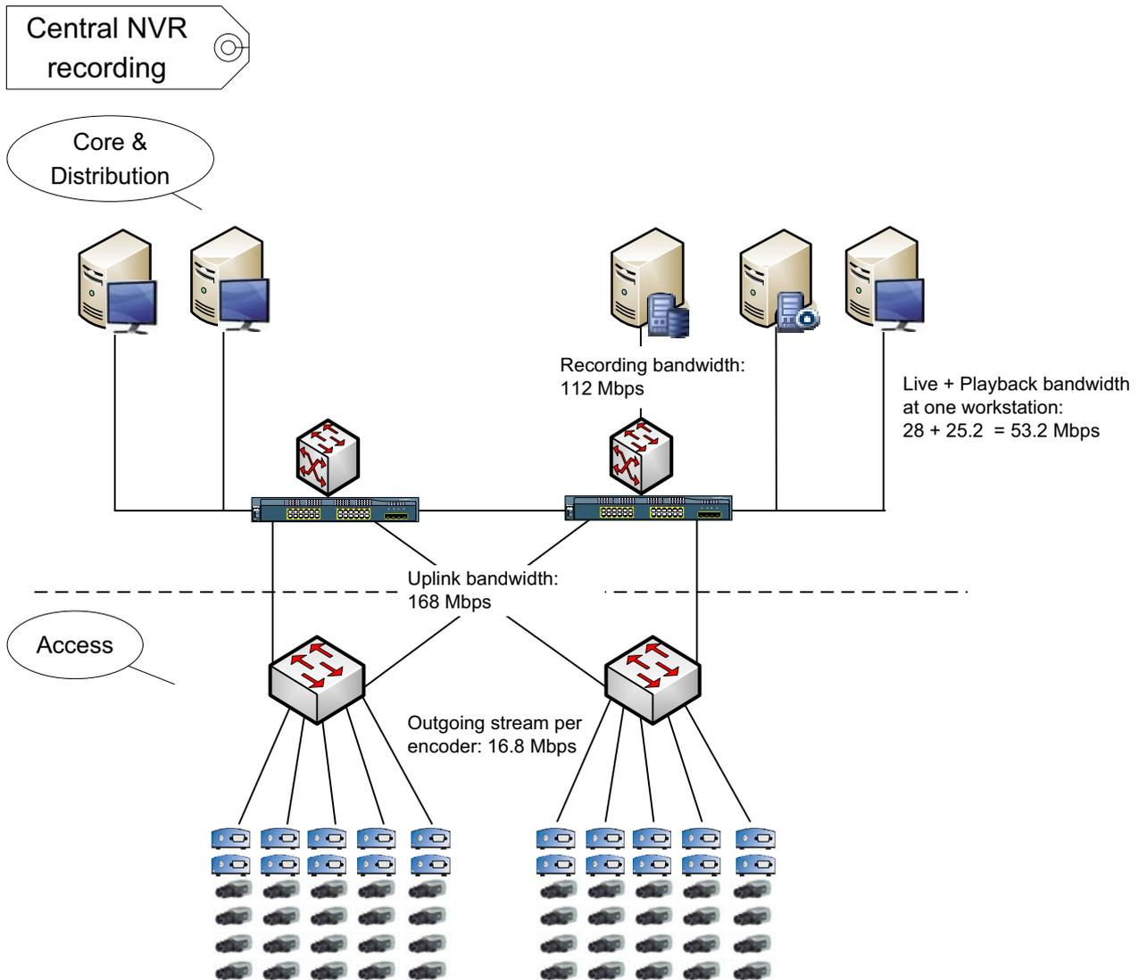
Figure 6.17 Central NVR recording
