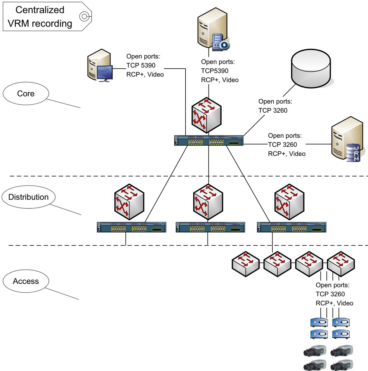
Figure 6.11 Centralized Bosch VMS VRM recording
