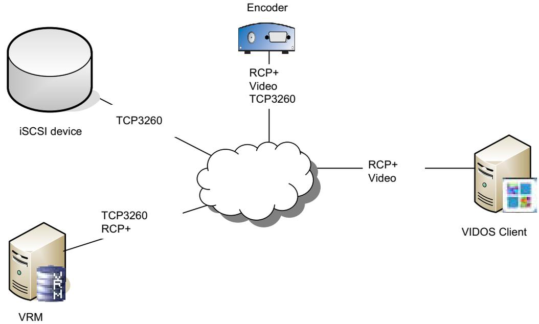
**Figure 6.10** Open ports for an encoder recorded via VRM and a VIDOS client
