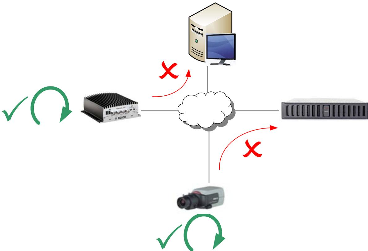
Figure 4.8 Recording at the edge
