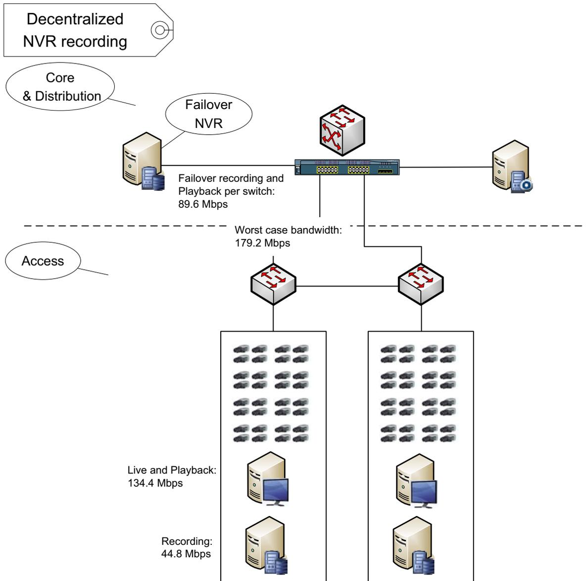
**Figure 6.26** Decentralized NVR recording
