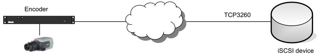
**Figure 6.5** Open ports for Direct-to-iSCSI recording
