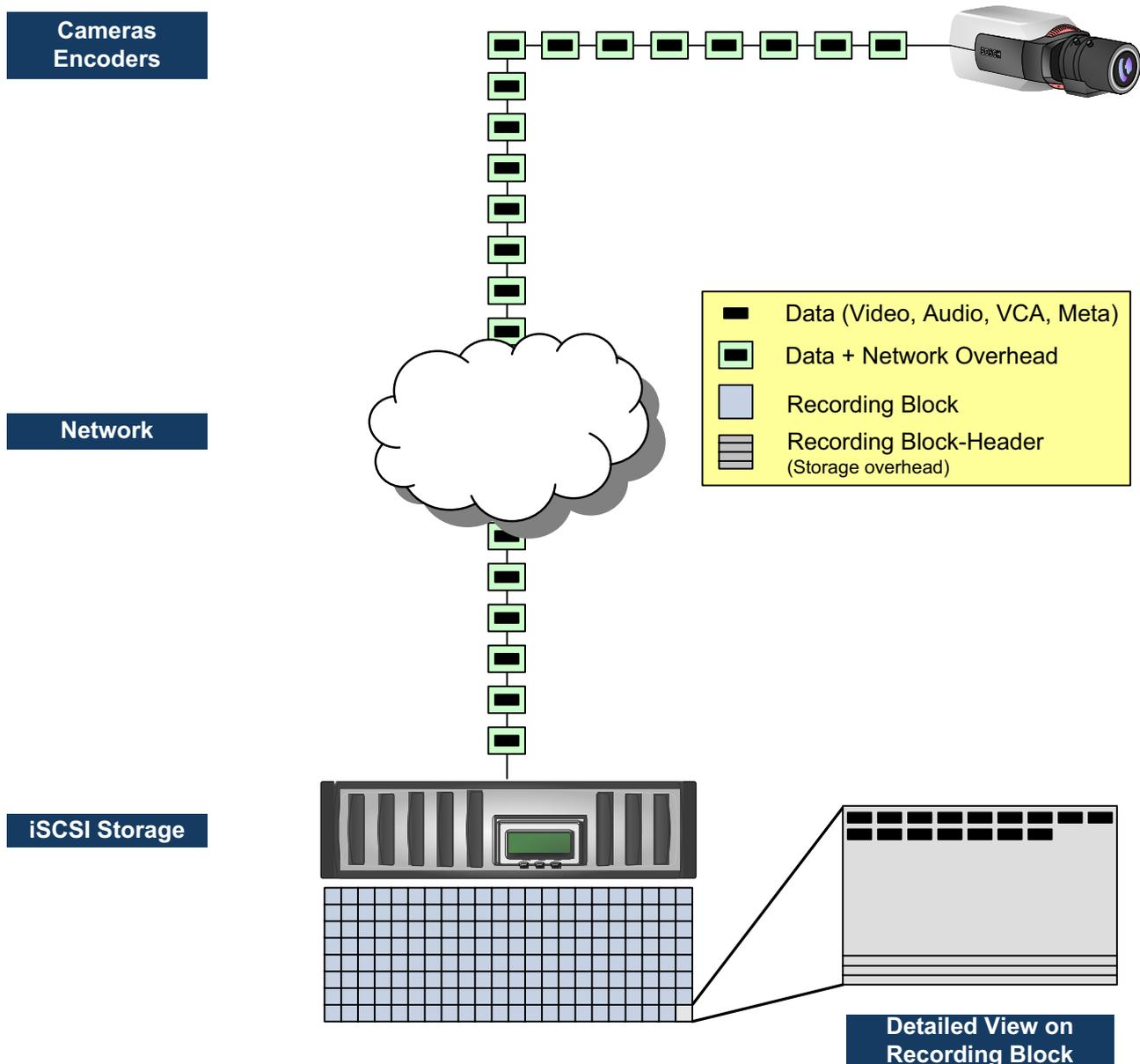
Figure 5.1 Relation between network bandwidth and storage calculation
