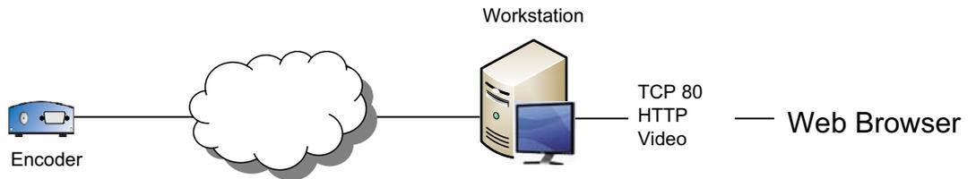
Figure 6.2 Open ports for Web browser connected to an encoder
