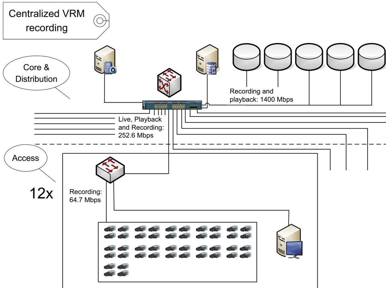
Figure 6.23 Centralized VRM recording
