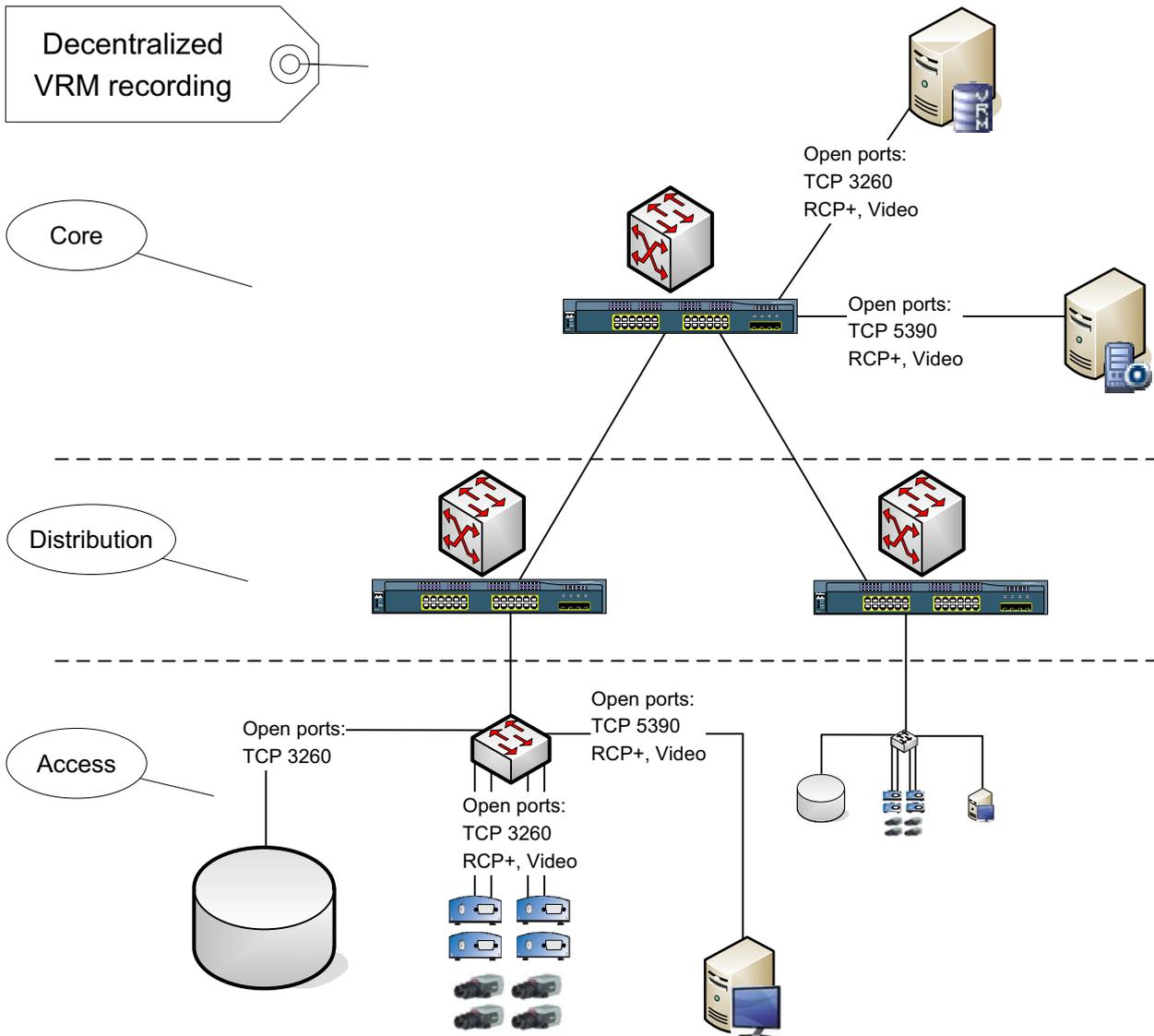
Figure 6.12 Decentralized Bosch VMS VRM recording
