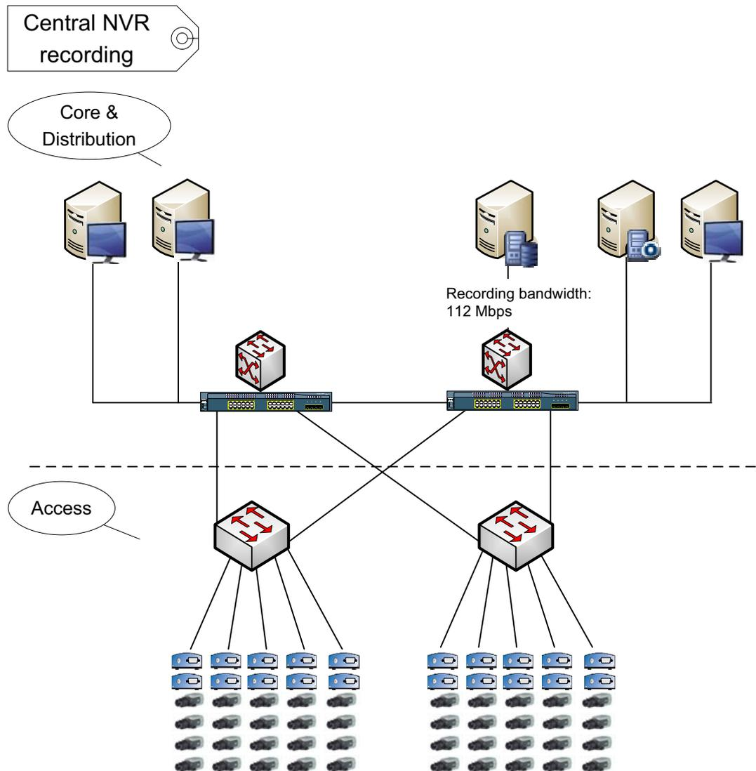
**Figure 6.18** Central NVR recording with export
