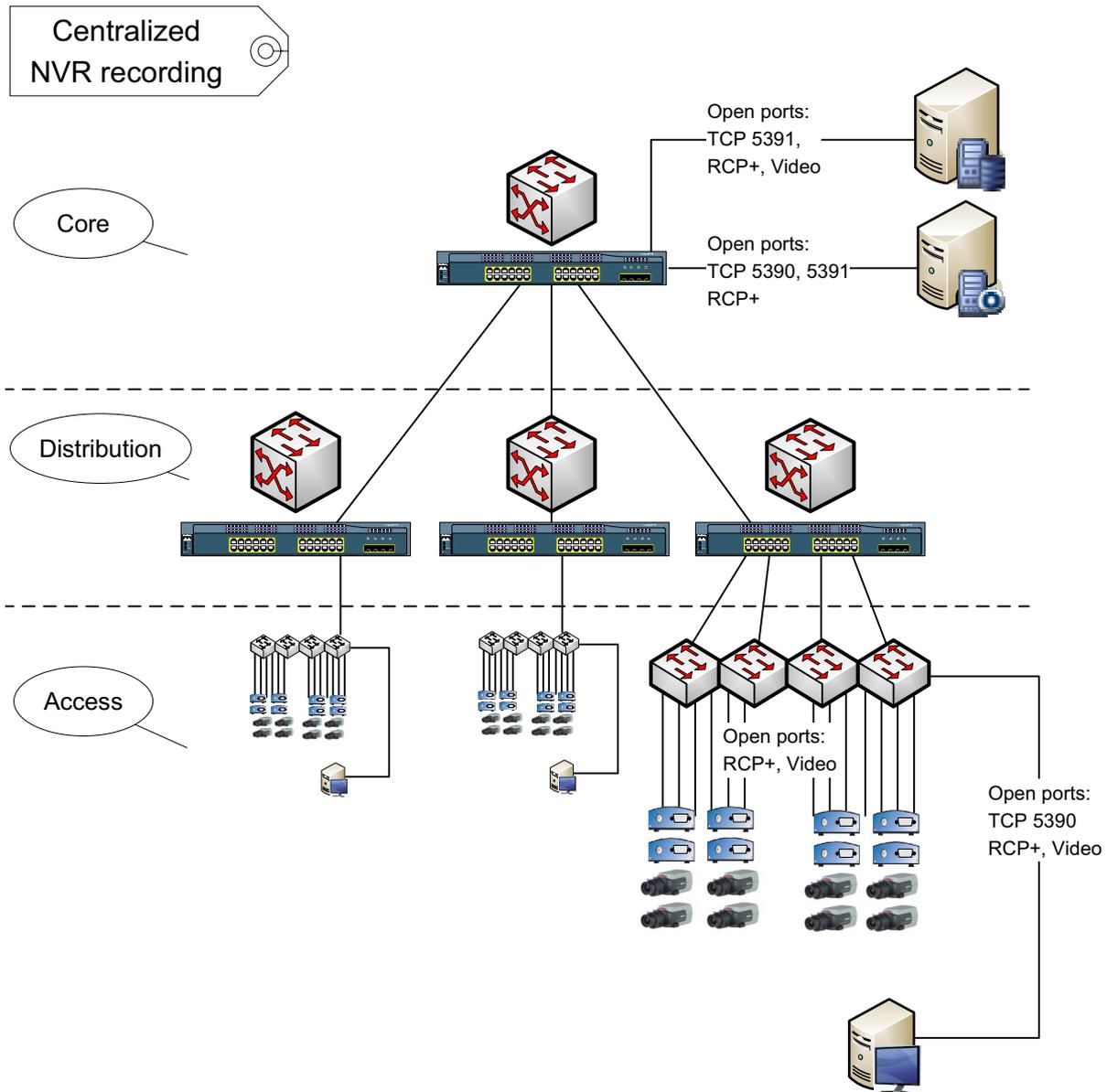
Figure 6.13 Centralized Bosch VMS NVR recording
