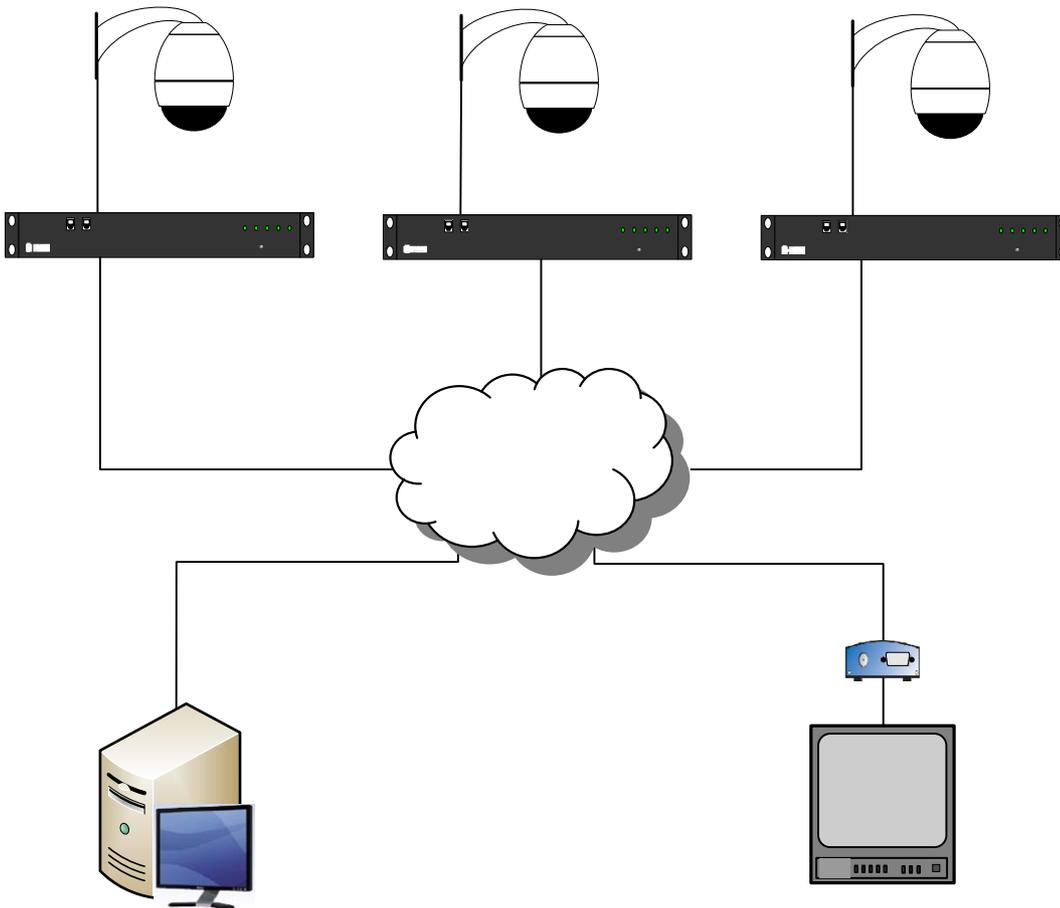
**Figure 2.4** Digital recording at the edge
