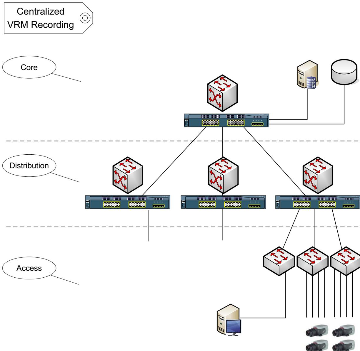
**Figure 3.3** Centralized VRM recording
