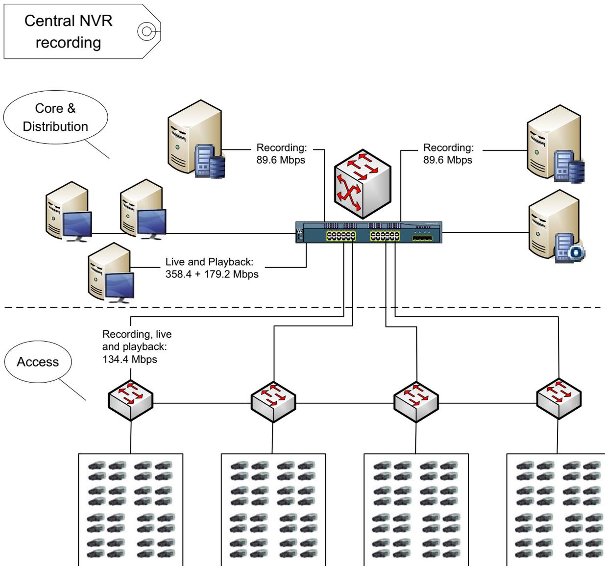
**Figure 6.25** Centralized NVR recording
