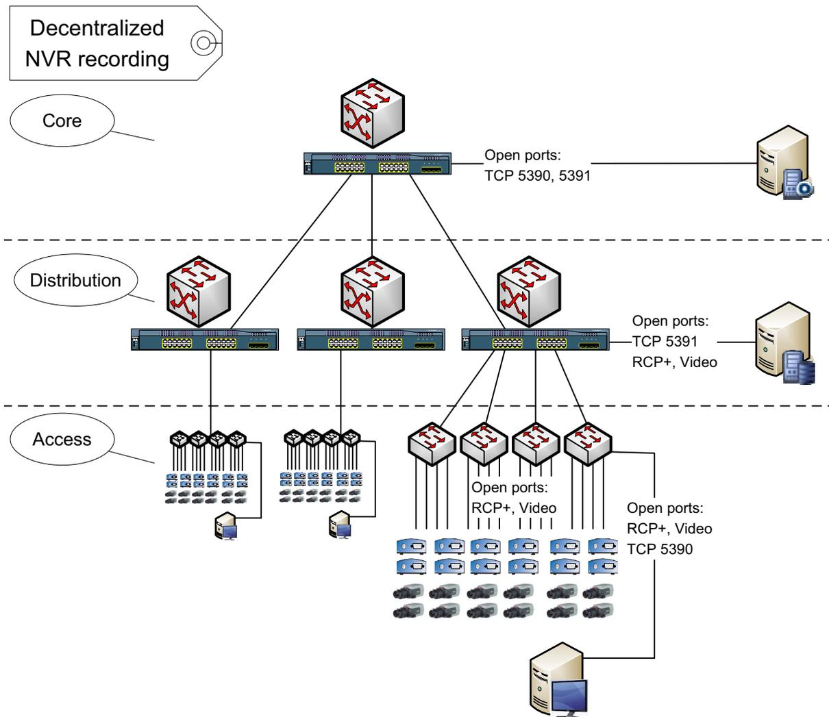
Figure 6.14 Decentralized Bosch VMS NVR recording
