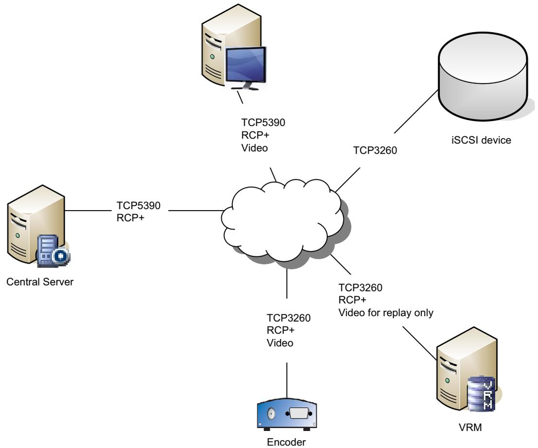
**Figure 6.7** Open ports for Bosch VMS recording with VRM
