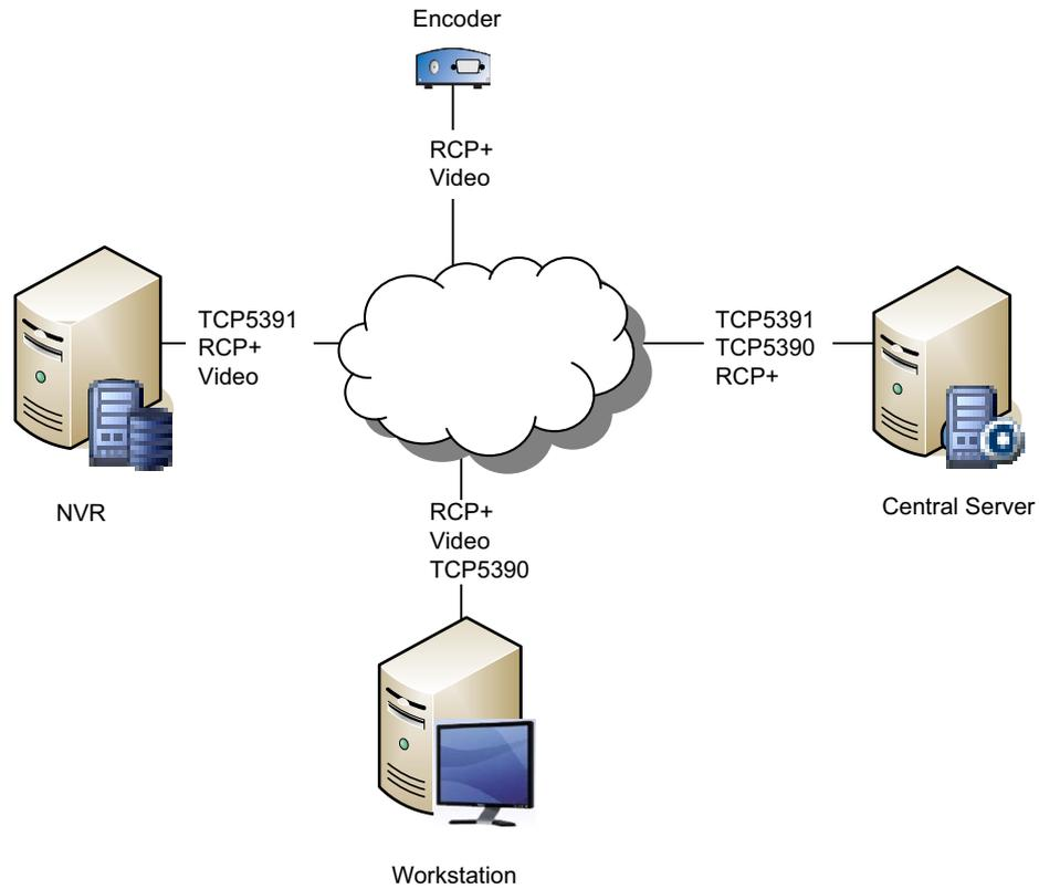
**Figure 6.8** Open ports for a Bosch VMS recording with NVR
