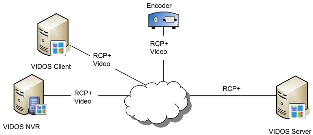
**Figure 6.9** Open ports for an encoder connected to a VIDOS system
