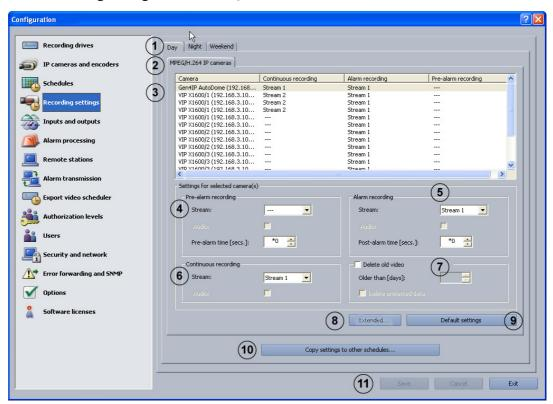
You can configure the recording settings for the MPEG4/H.264 IP camera in this dialog box.
