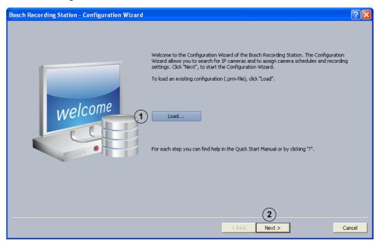
The configuration wizard allows you to search for IP cameras in the network and assign camera schedules and recording settings.
